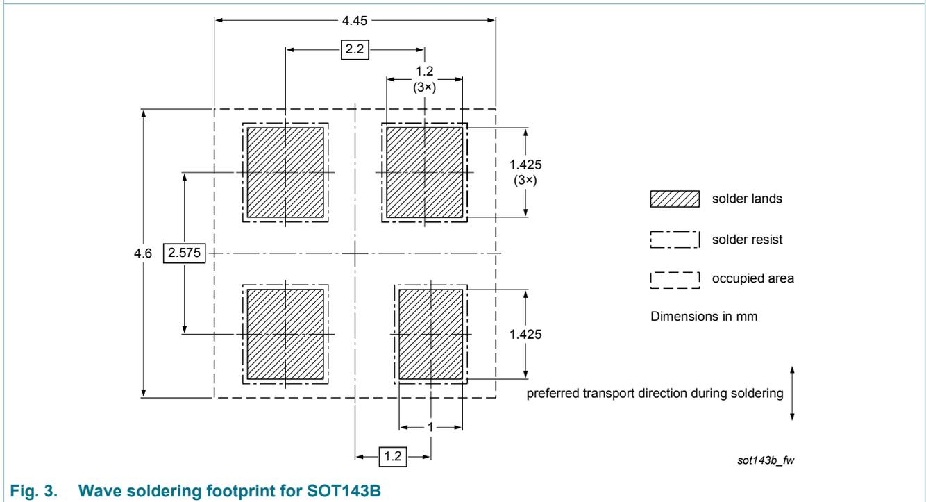
Fig. 3. Wave soldering footprint for SOT143B
