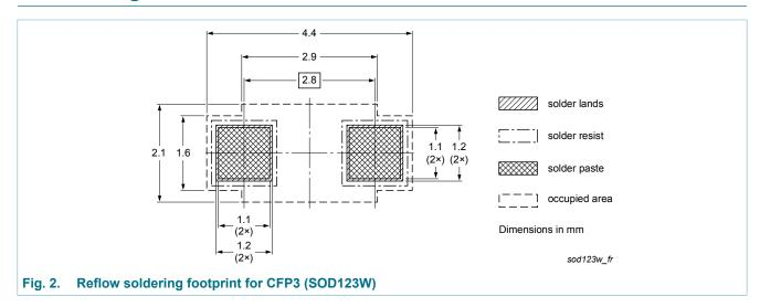
plastic, surface mounted package; 2 terminals; 2.6 mm x 1.7 mm x 1 mm body
