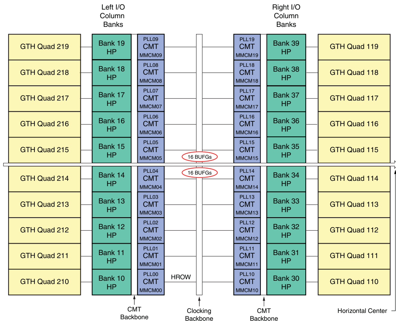
Figure 1-24: XC7VX690T and XQ7VX690T Banks
