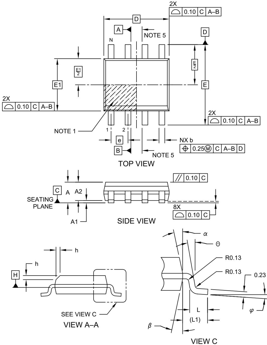
**8-Lead Plastic Small Outline (SN) - Narrow, 3.90 mm (.150 In.) Body [SOIC]**
