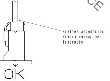
2) When applying load to connector end, please use the retainer for reducing the stress affection on the connector.
