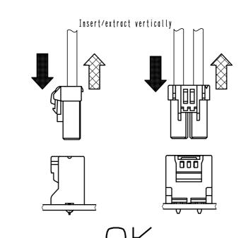
2) When it is hard to extract, please lightly insert the connector beforehand and then pull it with releasing the lock. Forced extraction has a risk of connector breakage.
