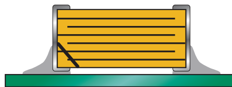
Type A: Angled crack between bottom of device to top of solder joint.
