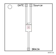
Max  $R_{\theta JA} = 160^{\circ}\text{C/W}$  when mounted on a minimum pad area of 2-oz (0.071-mm) thick Cu.
