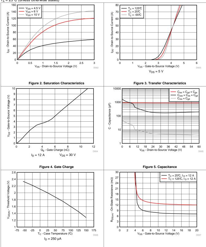
Figure 6. Threshold Voltage vs Temperature
