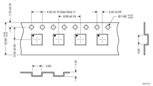
Notes: 1. 10-sprocket hole-pitch cumulative tolerance ±0.2.
