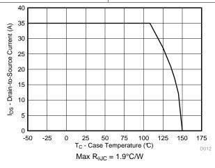
Figure 12. Maximum Drain Current vs Temperature
