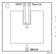
Max  $R_{\theta JA} = 55^{\circ} C/W$  when mounted on 1 in<sup>2</sup> (6.45 cm<sup>2</sup>) of 2-oz (0.071-mm) thick Cu.
