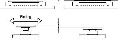
(2) WHEN GUIDING, THE CONNECTORS ARE ALIGNED PARALLEL TO EACH OTHER, WITH LONGITUDINAL AND LATERAL MOVEMENTS RESTRICTED. MATE THEM PROPERLY BY APPLYING FORCE IN THIS CONDITION.
