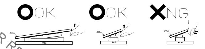
FPC IS NOT RIGID. THE CONNECTOR CAN BE BROKEN. PLEASE CHECK THE ACTION OF THE FPC TO BE USED REPEATERLY AT THE TIME OF TRIAL PRODUCTION. BE CAREFUL TO UN-MATE THEM FROM THE PITCH DIRECTION, DM THE CORNER CAN ALSO RISK TO PUTTING STRESS ON CONTACTS.
